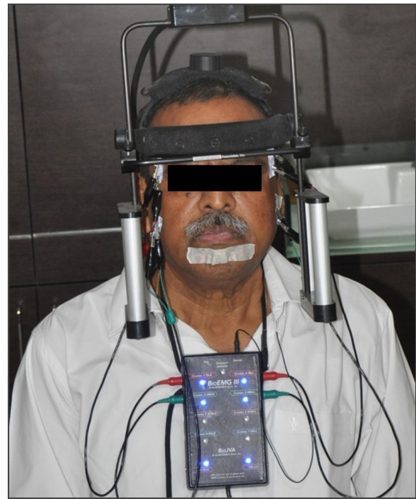
Figure 8. The JT-3D incisor-point tracker and BioEMG III amplifier applied to a potential reconstruction patient.
